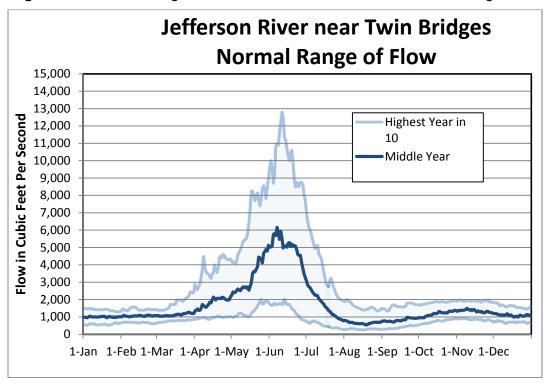
Figure 5.10 Normal Range of Flow for the Jefferson River near Twin Bridges
