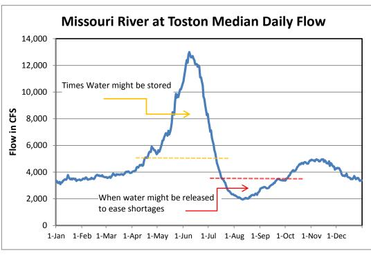
**Figure 9.1** Example flow graph for the Upper Missouri Basin depicting times of potentially storable flow and when releases might be used to offset shortages.
