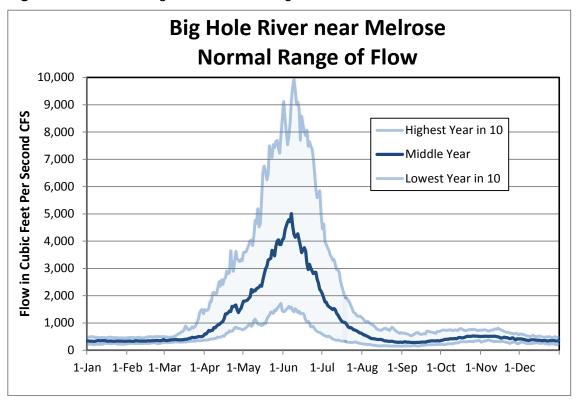
Figure 5.9 Normal Range of flow for the Big Hole River near Melrose
