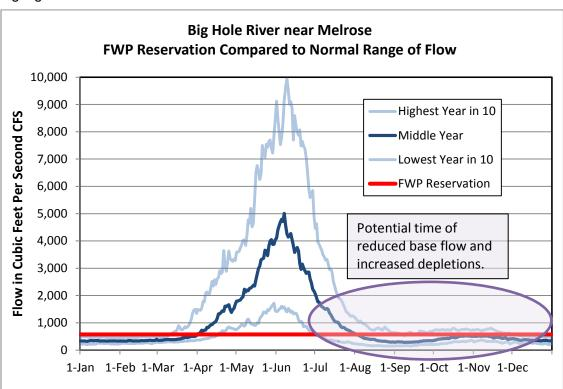
Figure 8.5 Big Hole River flow graph with times when lower minimum flows are projected highlighted
