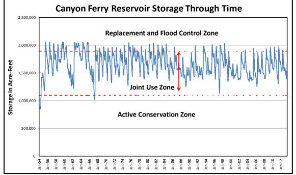
Figure 6.38 Canyon Ferry Reservoir storage from date of dam construction to near present
