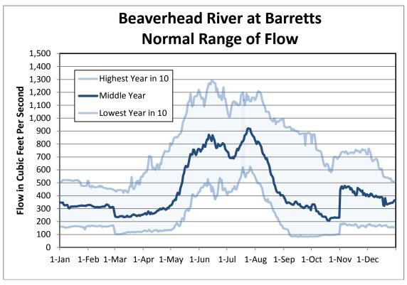
Figure 5.8 Normal range of flow for Beaverhead River at Barretts
