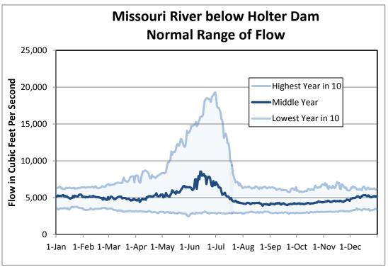
Figure 5.13 Normal Range of flow for Missouri River below Holter Dam
