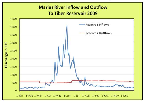
Figure 6.39 Flows upstream and downstream of Tiber Reservoir during 2009
