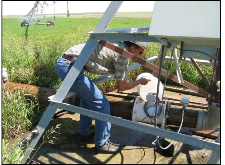
Photos 1 and 2. Pipe flow meters on the Berkram and Smrcka Sprinkler Irrigation Systems.
