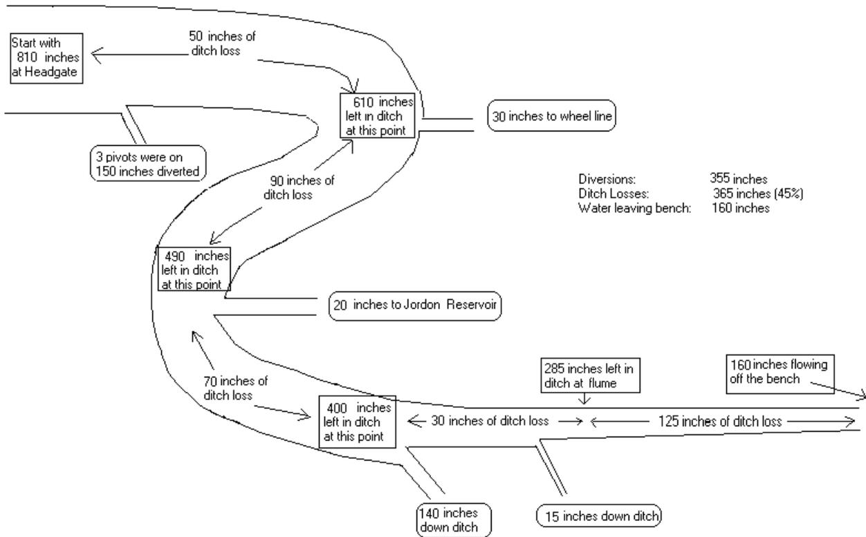
Big Ditch Flow Partial Flow Balance Diagram for July 1, 2003
