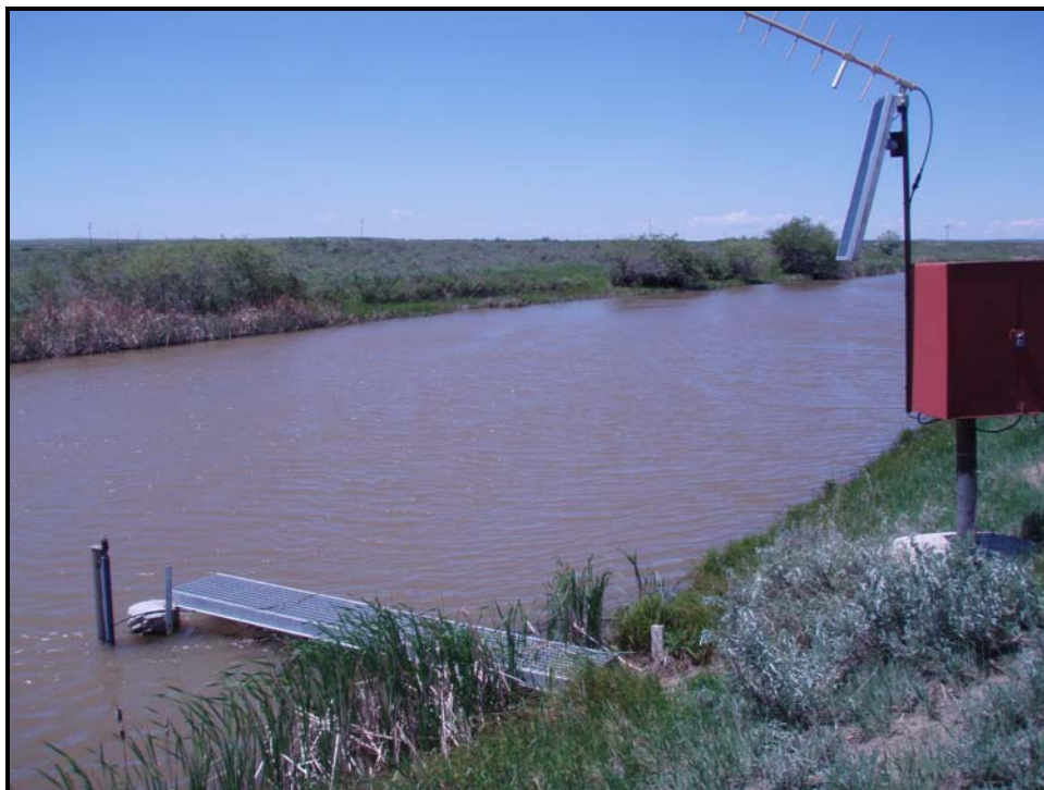
Photo 10.4 - Hydromet flow monitoring Station on the Dodson South Canal. Photo: Larry Dolan
