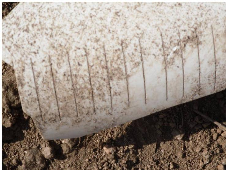
Figure 11 - Plugged Drain Pipe Slots
