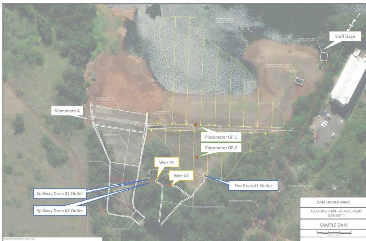
Figure 2.1 – An example plan drawing showing the location and name of all instruments at a dam.
