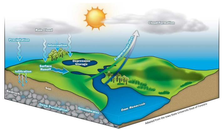
Figure 1. Total rainfall-runoff process with losses
