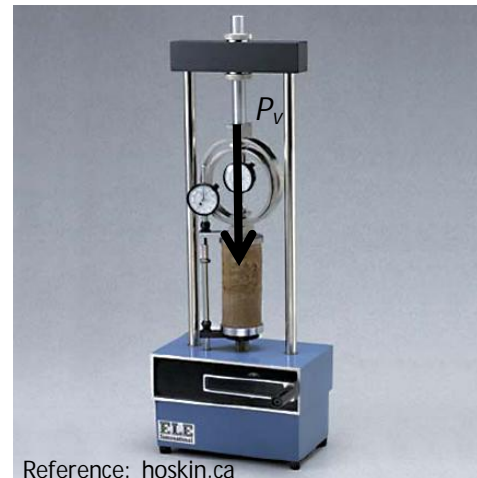
Figure 4: Unconfined compression test apparatus.
