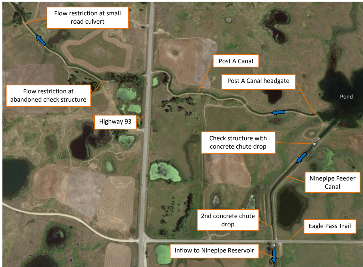
Figure 46. Existing control near the head of the Post A Canal
