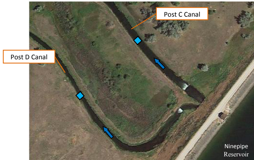
Figure 65. Approximate location of possible new Replogle flumes at the head of the Post C and D Canals
