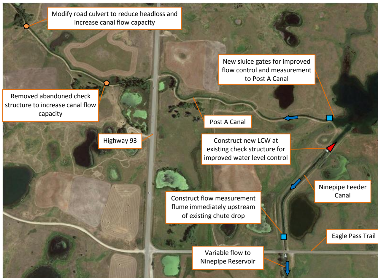
Figure 50. Improvements near bifurcation of Ninepipe Feeder Canal and head of the Post A Canal
