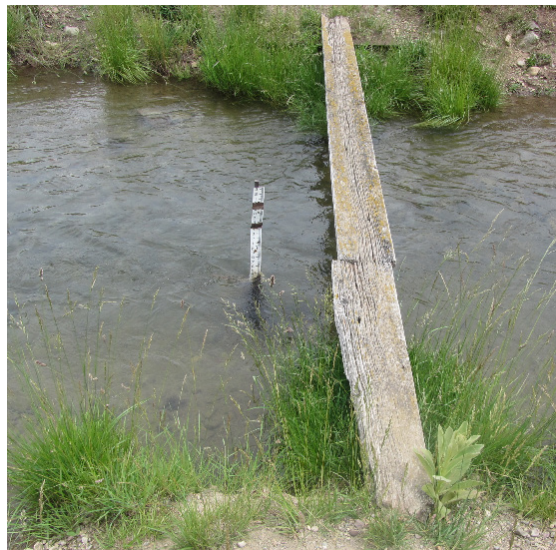
Figure 33. GOES gauging station for flow measurement downstream of the Mission B Canal headgates
