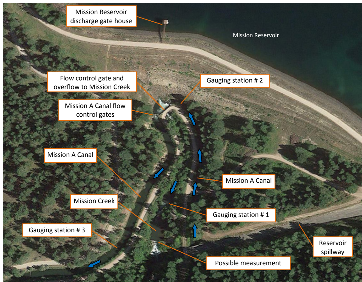
Figure 14. Overview of existing control at the discharge of Mission Reservoir
