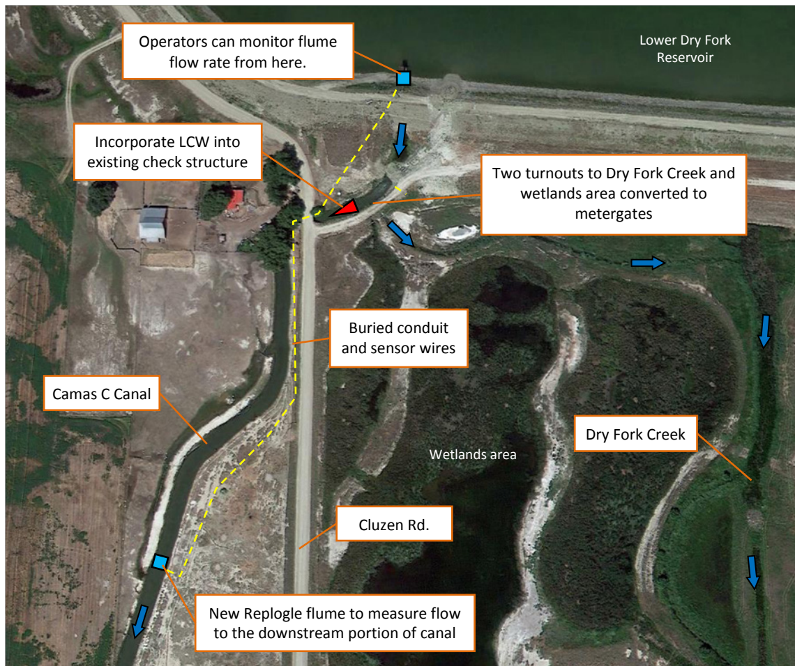
Figure 31. Control improvements at the head of Camas C Canal and Lower Dry Fork Reservoir discharge
