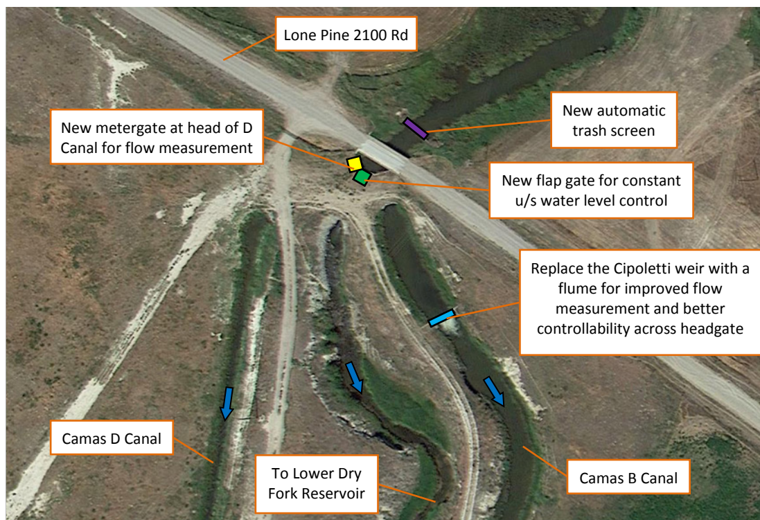
Figure 26. Improvement changes at the Camas B and D Canal headgates
