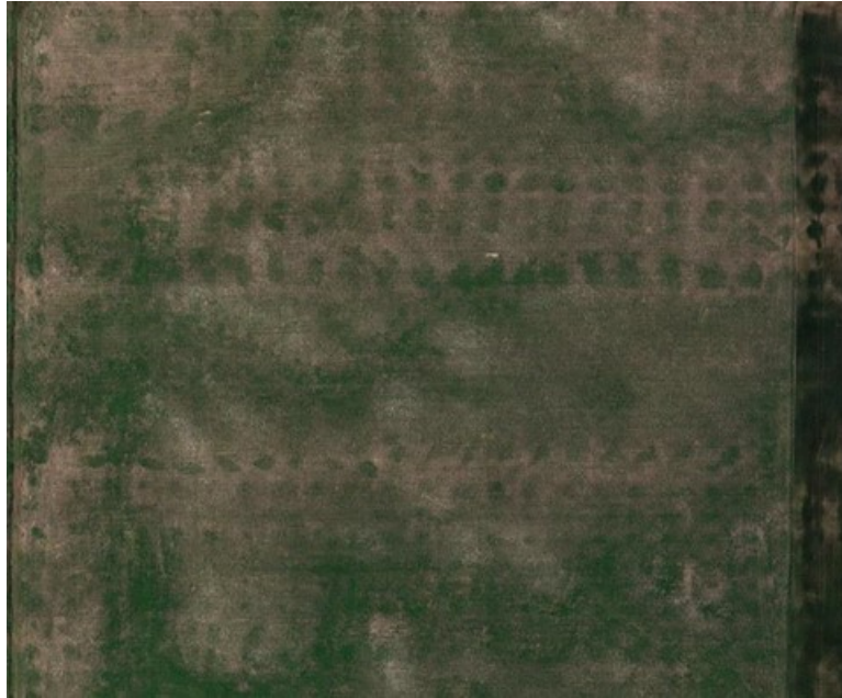
Figure 1. The district circular patterns of uneven crop growth are caused by a poor side roll sprinkler system DU
