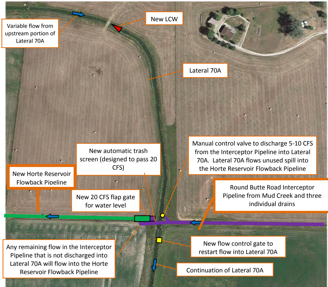
Figure 36. Modernization components of the Lateral 70A Pool
