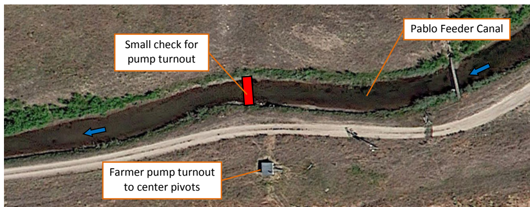
Figure 21. Approximate location for new Pump Station #2 on the Pablo Feeder Canal
