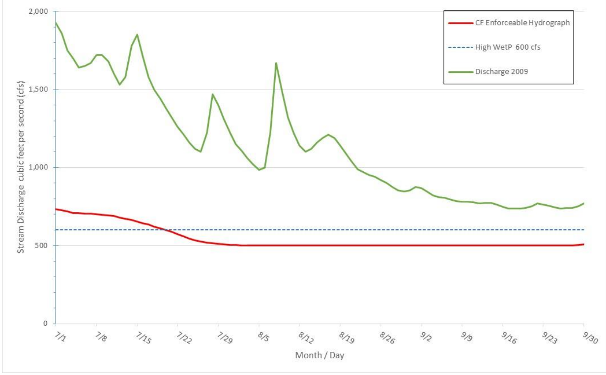
2009 Clark Fork River Daily Stream Flow @ Turah, Mt Compared to Milltown Instream Water Right
