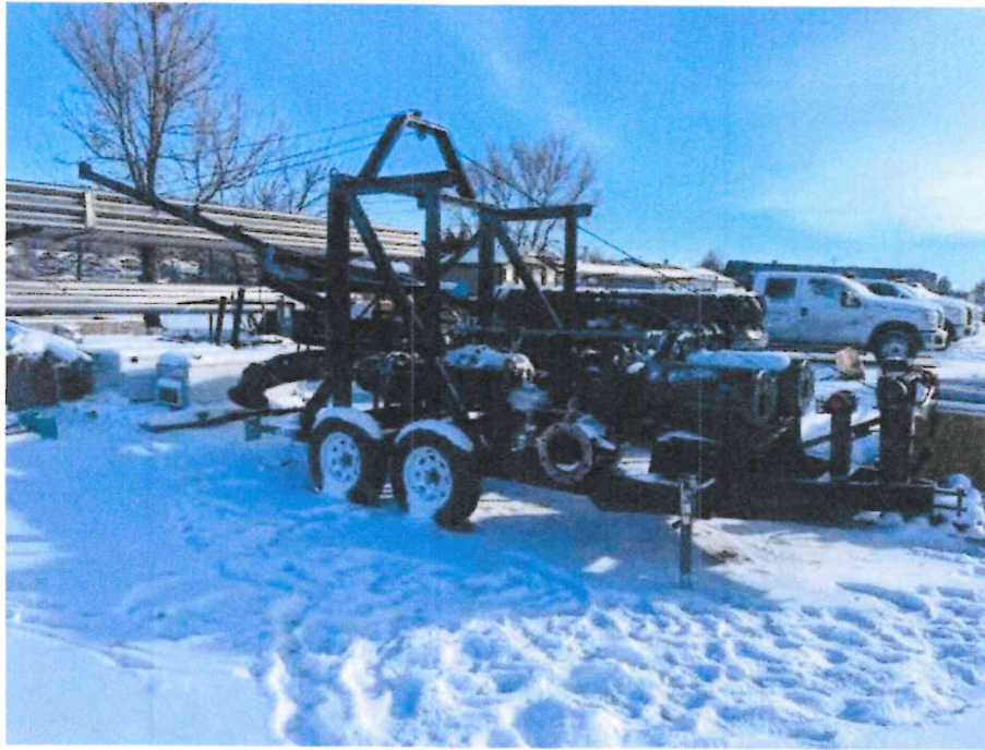
Figure 7: Example of mobile pumping station that will be used at both proposed POD locations, picture provided by Scott Swenson, Big Sky Irrigation.
