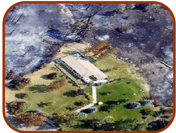
Defensible space around a home is not a guarantee of success but it does increase the odds of a home being able to withstand the combined effects of wildfire.
