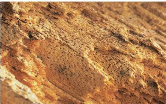
Figure 128. Decay from laminated root rot has distinctive, pinhead-sized round pits.
