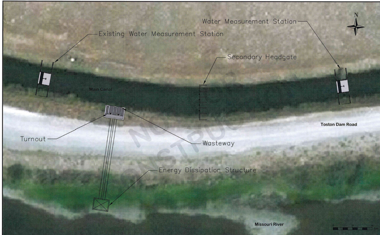
Figure 5: Conceptual Layout of Broadwater-Missouri Canal Improvements
