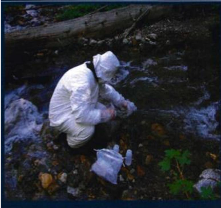
Trace chemistry measures amounts of chemicals in such small concentrations that clean gear and clean procedures are required
