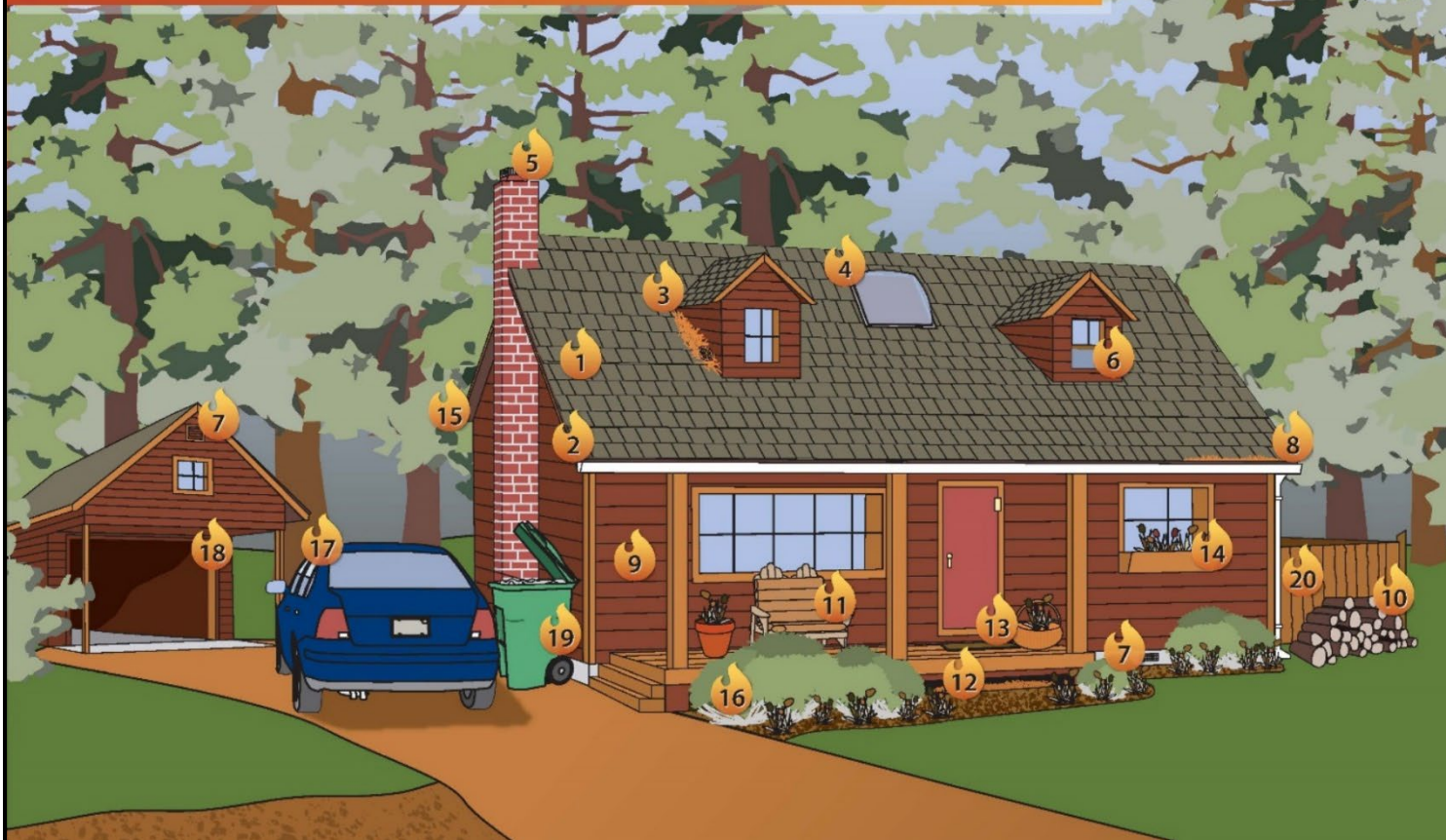
Figure 3.4. An example home in the WUI with ember ignition hazards identified by numbered flames.
