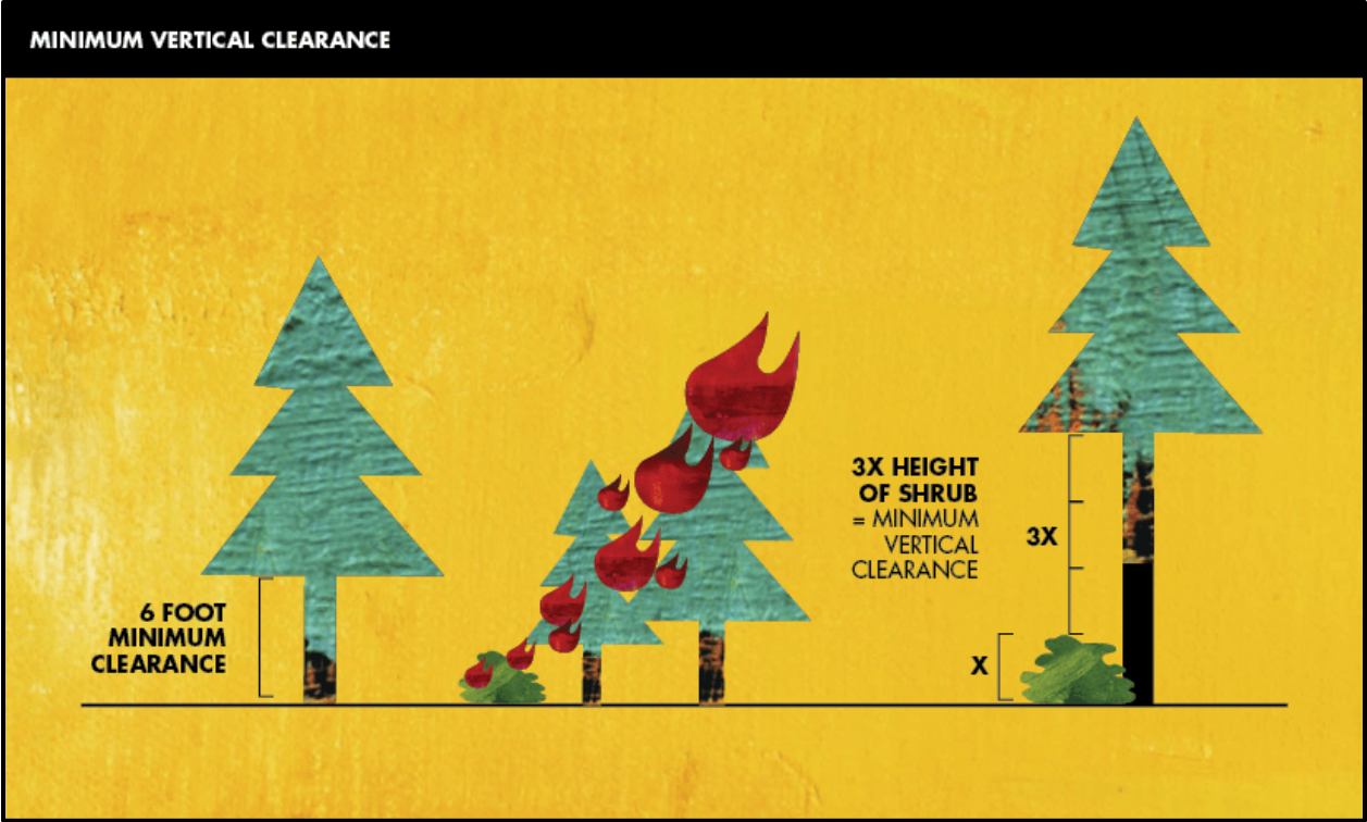
Figure D.3. Recommended minimal vertical clearance.
