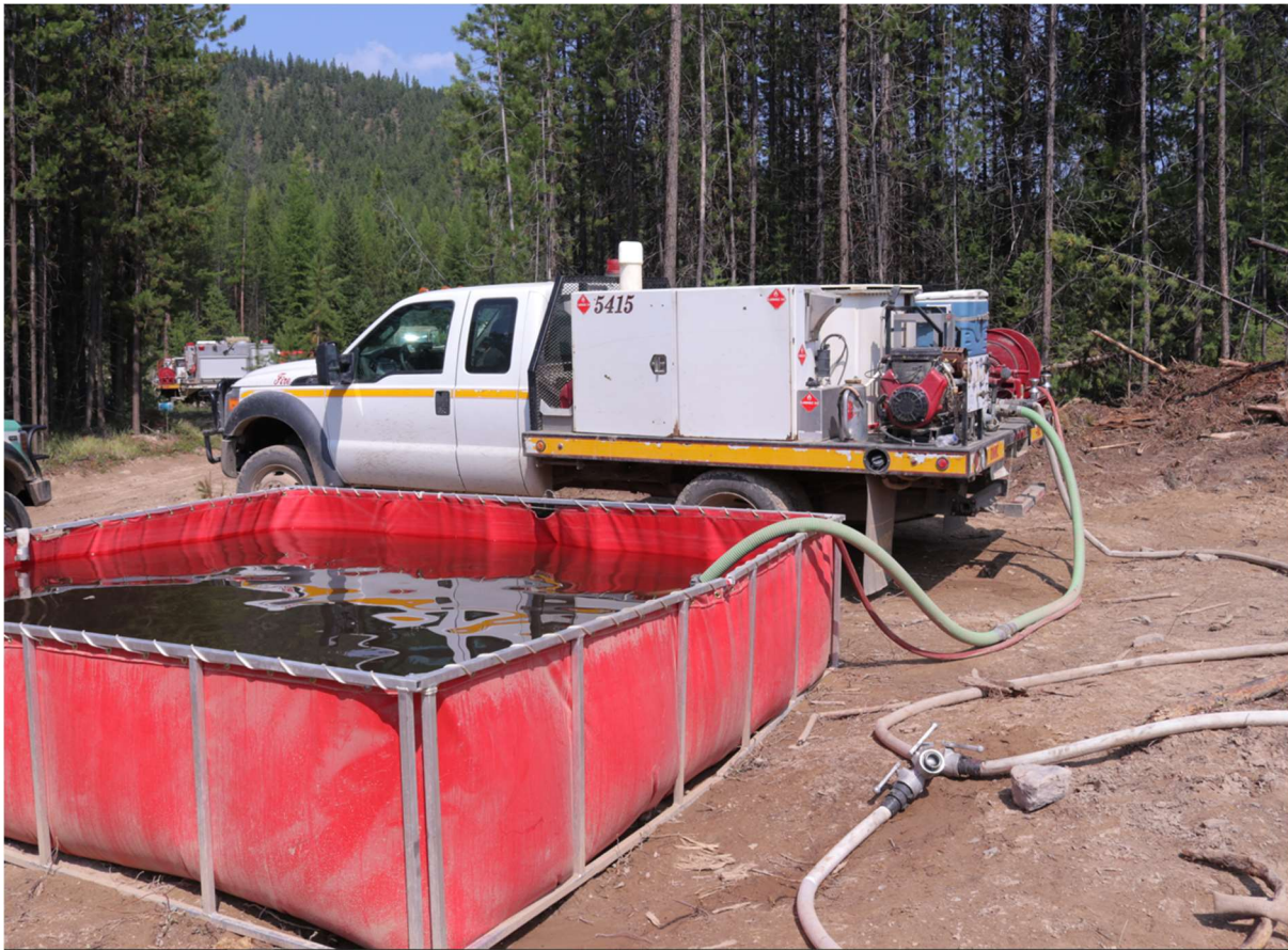
DNRC engine pumping from a Port-A-Tank with a hose lay setup
