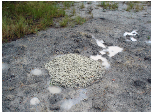
Improperly abandoned dry well
