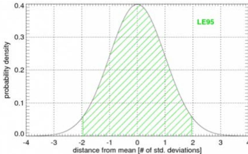
Figure 10. Normally distributed error, with the shaded area corresponding to LE95 or 95% confidence interval covering 95% of the area under the Gaussian Curve
