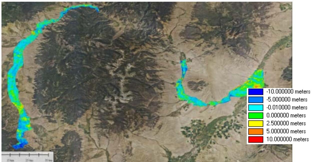
Figure 8. NEXTMap DTM minus NED Difference Surface Overlaid on the NAIP Imagery
