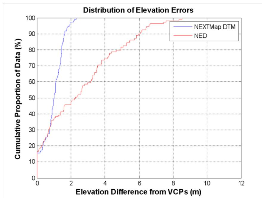
Figure 6. Cumulative Distribution of Errors for NEXTMap DTM and NED
