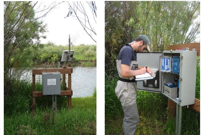
The measurements happen automatically about every 15 minutes, and that data is sent out once an hour to a satellite that transmits it to the network's hub computers. Most real-time stream gages in Montana, use a pressure sensing device to determine the river stage. The benefit of these systems is that they are highly accurate and maintain consistent records with low maintenance.
