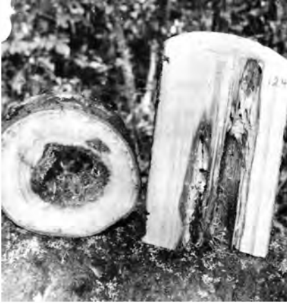
Figure 2.—Cross and longitudinal sections showing advanced stages of white butt rot caused by Armillaria mellea . Stereum chailletii , another white rotter, was isolated from the faint discolored streaks, seen in both sections, in the wood between the A. mellea rot and the bark.
