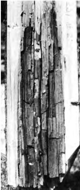
Figure 3.— Polyporus balsameus : Left, A typical brown cubical rot in balsam fir; right, fructing bodies of the fungus on rotted sections.
