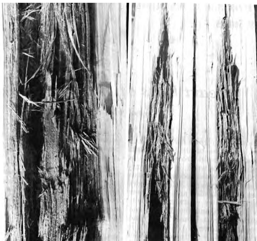
Figure 1.—White butt rots in balsam fir bolts: Left , Caused by Poria subacida ; right , caused by Odontia bicolor . Note the stringiness of the rotted wood.
