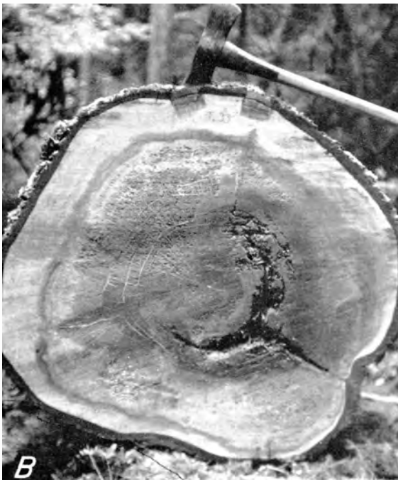
Figure 2.—Typical brown rots in western hemlock: A, Shattered log showing longitudinal view of advanced decay in the heartwood caused by the velvet top fungus; B, cross section of a log showing advanced and incipient stages of decay caused by the sulfur fungus; C, tangential section of advanced decay (above) and radial section (below) showing advanced and incipient stages of decay caused by the red belt fungus.
