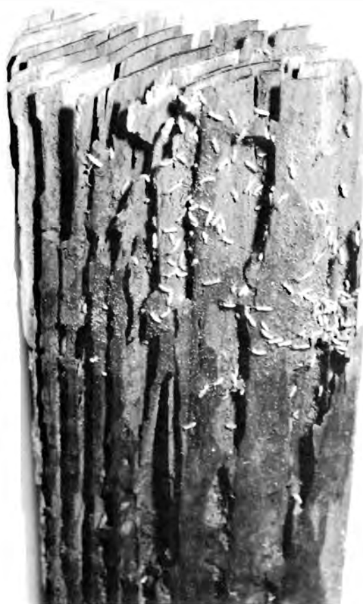
Figure 3.—Pine 2x4 destroyed by termites.
