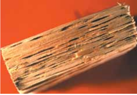
Figure 9. Advanced decay caused by the coral fungus showing the long, spindle-shaped pockets, or pits, with firm wood in between.
