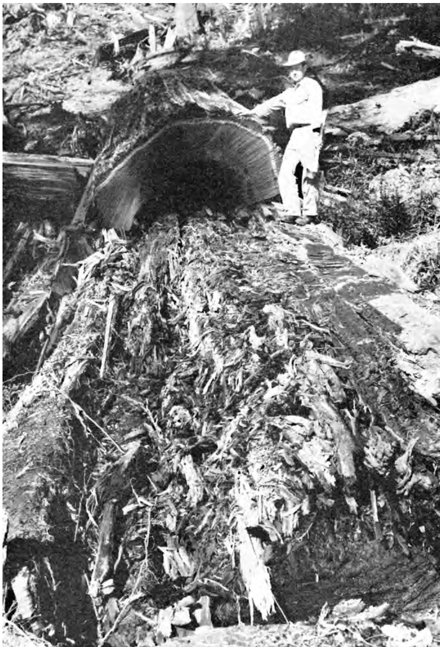
FIGURE 4. —White ring rot of redwood caused by Poria albipellucida : Longitudinal view of badly decayed log, showing stringy nature of the rot.
