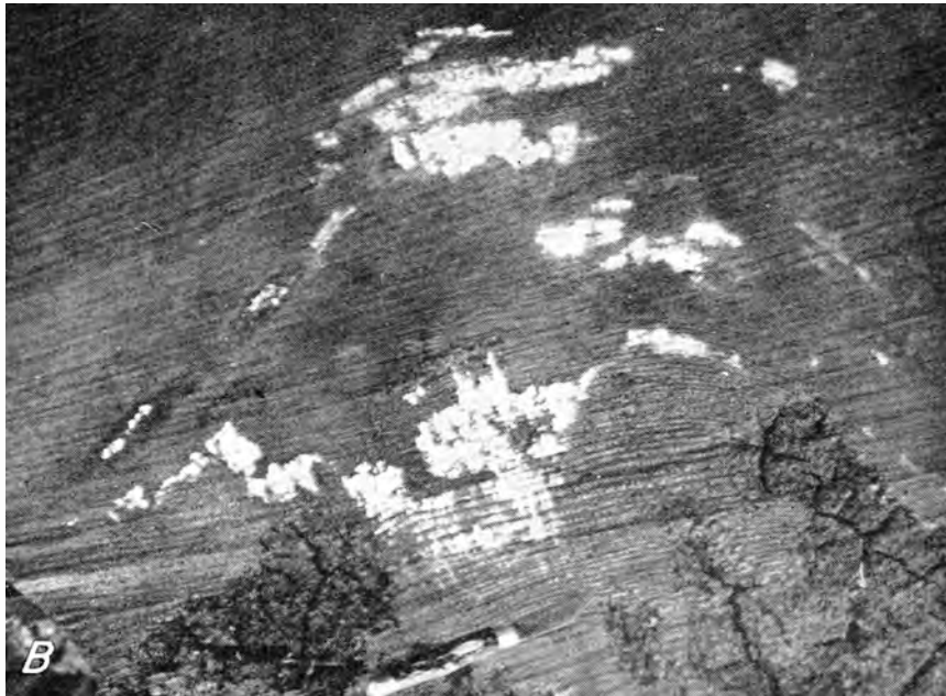
FIGURE 2.—Brown cubical rot of redwood: A, Longitudinal detail of rot pockets in a split log; B, fruiting of the fungus on the end of a decayed log.
