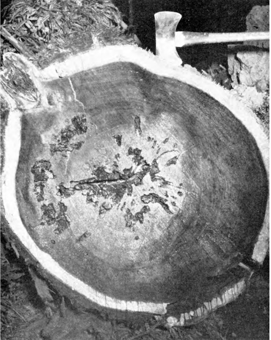
FIGURE 1. —Brown cubical rot of redwood caused by Poria sequoiae : End of an old-growth log showing a cross section of rot pockets.
