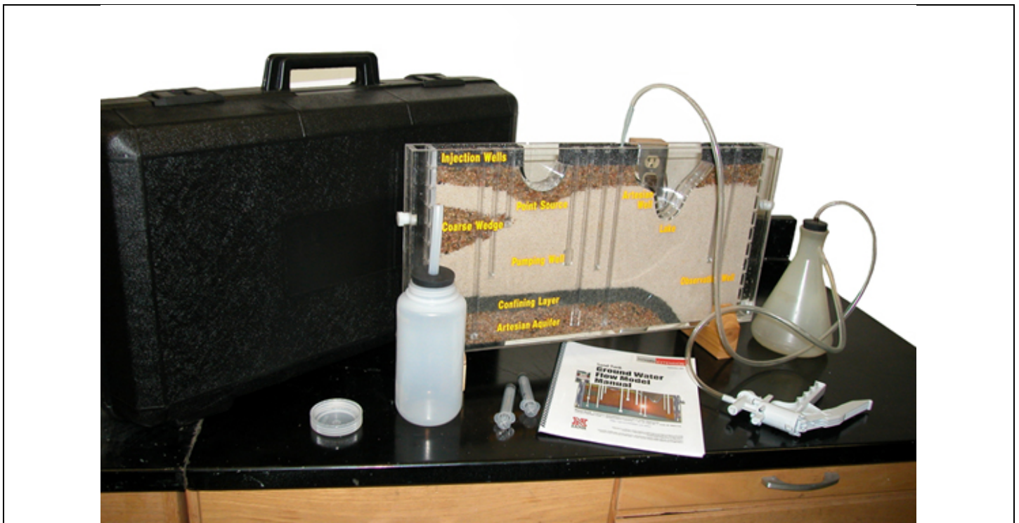
Sand-Tank - Ground Water Flow Model and plastic storage case.
