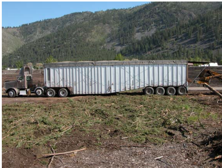
Figure 13. 148 cubic yard capacity chip vans were also used in the study. They could only haul about 34 tons (green) of product due to legal maximum weight restrictions.
