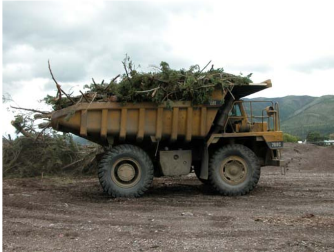
Figure 8. Slash was also hauled in a Caterpillar Model 769C off-highway dump truck (31.7 CY, rated 36 tons max.).
