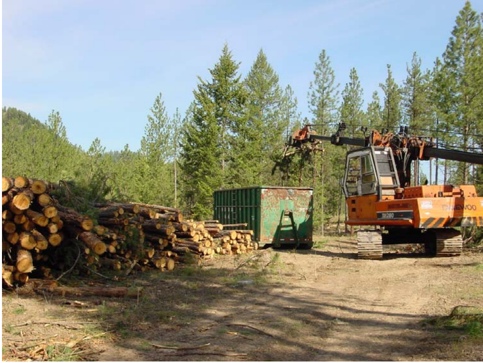
Figure 17. Daewoo DH280 with Denis strokeboom delimeter loading slash into roll on/off container.
