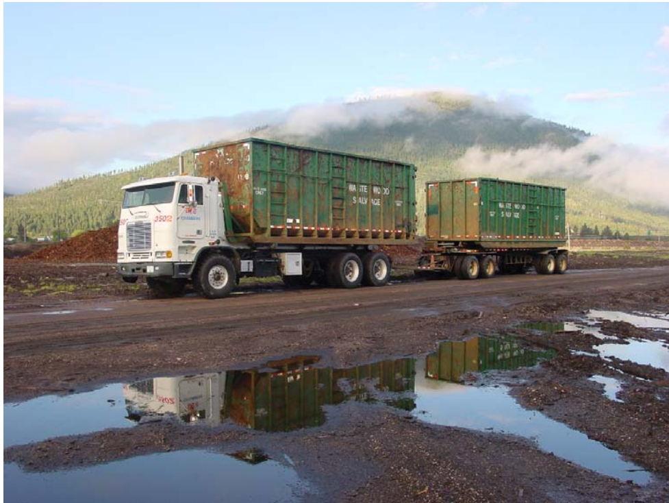
Figure 14. Roll on/off container truck system complete with roll on/off pup trailer.
