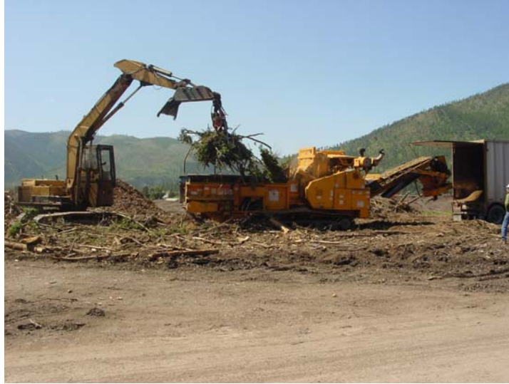
Figure 12. Grinding operation at Stimpson mill yard. A Komatsu log loader was used to feed a Bandit Model 3680 Beast recycler. The Beast had an optional 62-hp centrifuge blower to load chips. “Hog fuel” was blown directly into either a chip van or roll on/off container truck with pup trailer.
