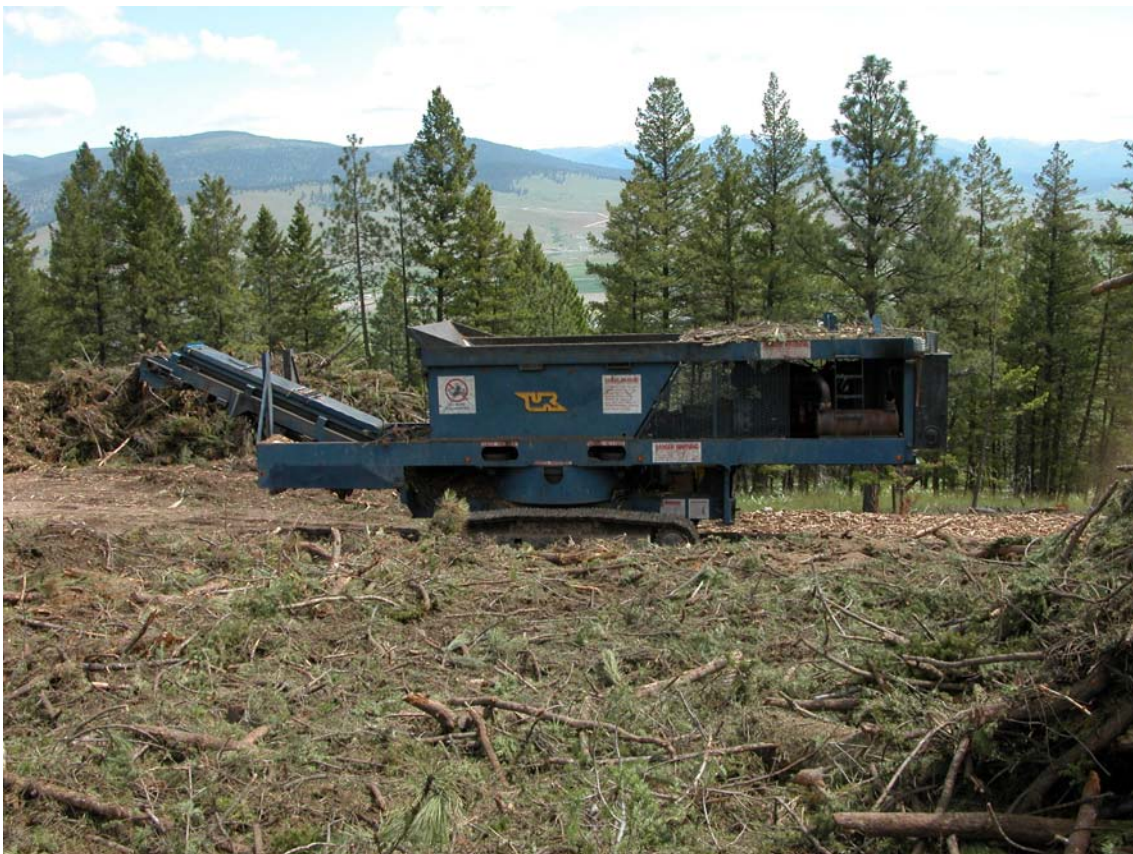
Figure 2. At the Dry Creek study site, the grinder was a modified Universal Refiner PDR-80-63, 475-hp grinder with conveyor belt. The unit was converted to radio control and set on tracks. The loader operator controlled both the loader and the grinder.
