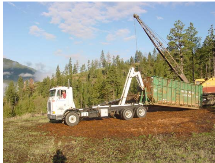
Figure 7. Loading roll on/off container for transport. The roll on/off container truck system used in the study was a cabover Freightliner tractor (430 hp) with a Stellar Industries hooklift conversion and a pup trailer. The roll on/off containers had a capacity of 48 cubic yards each. This system was leased from DCT Chambers of Vernon, British Columbia.
