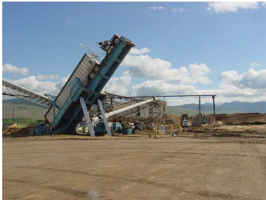
Figure 15. Chip van being unloaded at Smurfit-Stone. Roll on/off container truck unloading in the background.
