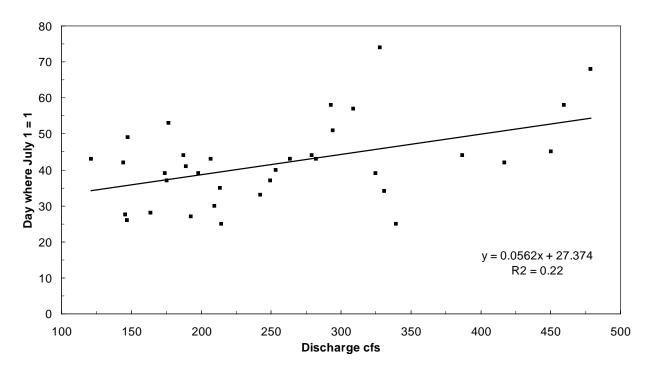
Figure 7. Middle day of 15 day lowest mean flow (where July 1 = 1) versus yearly average discharge (p < 0.01) based on data from the USGS Deer Lodge gage from 1979 to 2013.
