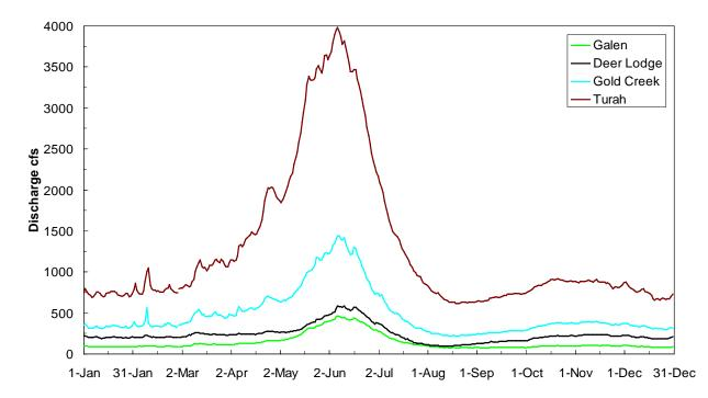
Figure 11. Average daily discharge from 1988 to 2013 at four USGS gaging sites on the UCFR.
