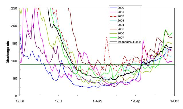
Figure 10. Discharge versus date for each year from 2000 to 2007 based on data from the USGS Deer Lodge gage with associated lower inflection point.
