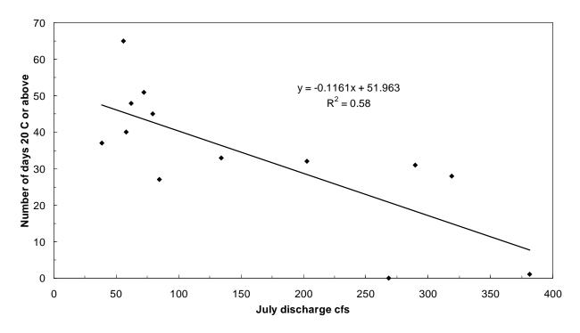
Figure 4. Relationship between annual number of days 20 C or above and July mean monthly discharge (p < 0.01) based on USGS Galen data from 1992 to 2004.
