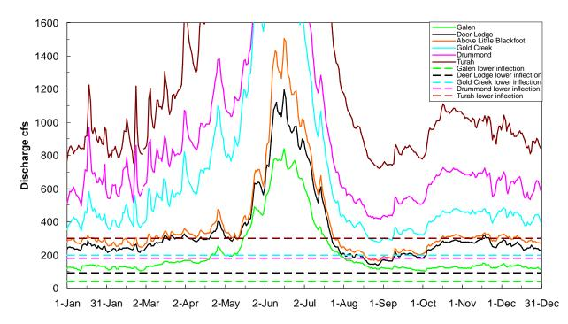
Figure 14. Average daily discharge from 2010 to 2012 (moderately high discharge) at six USGS gaging sites on the UCFR with lower inflection points associated with each gaging station.
