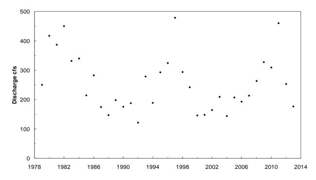
Figure 8. Yearly average discharge versus year based on data from the USGS Deer Lodge gage from 1979 to 2013.
