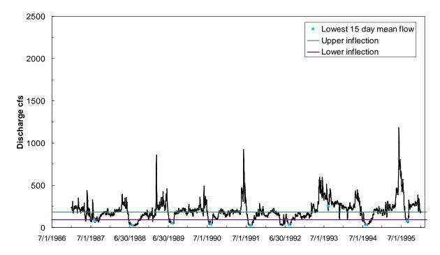
Figure 2. Daily discharge versus time at the USGS Deer Lodge gage from 1987 to 1995.
