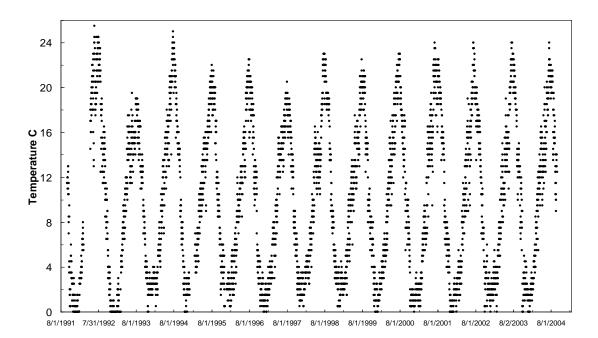
Figure 2. Maximum daily temperatures versus date based on USGS data from the Galen gage from 1991 to 2004.
