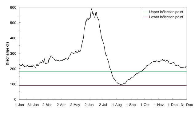
Figure 5. Average daily discharge versus time at the USGS Deer Lodge gage from 1978 to 2014.
