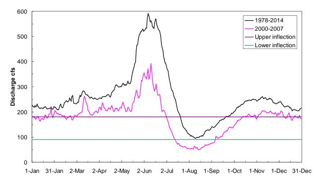
Figure 9. Yearly average discharge versus year based on data from the USGS Deer Lodge gage from 1978 to 2014 and 2000 to 2007.
