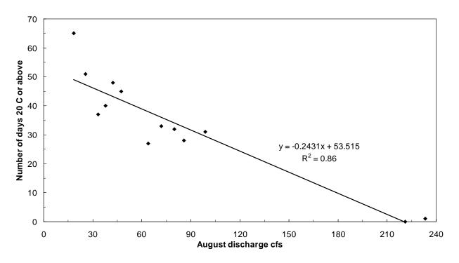
Figure 5. Relationship between annual number of days 20 C or above and August mean monthly discharge (p < 0.01) based on USGS Galen data from 1992 to 2004.
