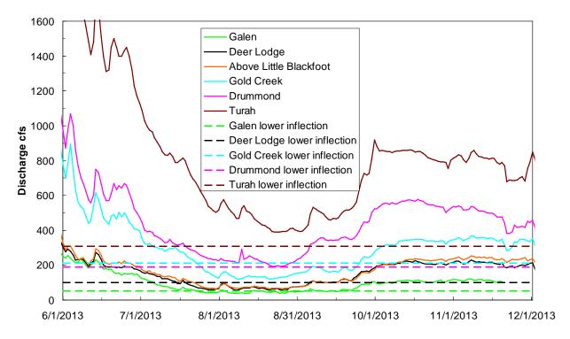
Figure 17. Daily discharge from 2013 (low flow year) at six USGS gaging sites on the UCFR with lower inflection points associated with each gaging station.
