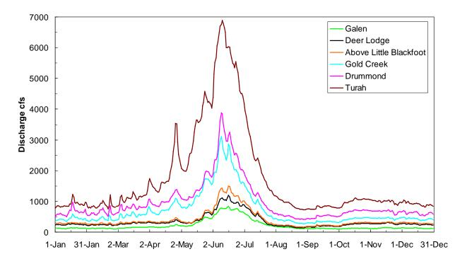
Figure 13. Average daily discharge from 2010 to 2012 (moderately high discharge) at six USGS gaging sites on the UCFR.
