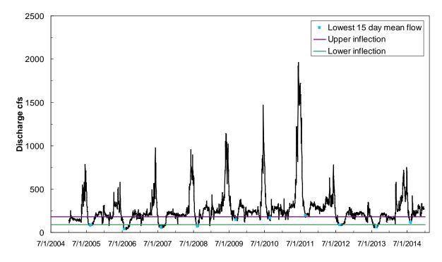
Figure 4. Daily discharge versus time at the USGS Deer Lodge gage from 2005 to 2014.
