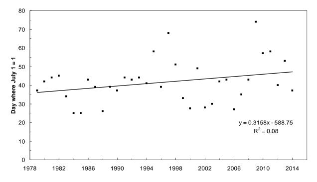
Figure 6. Middle day of 15 day lowest mean flow (where July 1 = 1) versus year (p = 0.09) based on data from the USGS Deer Lodge gage from 1979 to 2014.
