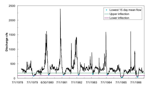
Figure 1. Daily discharge versus time at the USGS Deer Lodge gage from 1978 to 1986.
