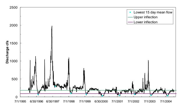
Figure 3. Daily discharge versus time at the USGS Deer Lodge gage from 1996 to 2004.
