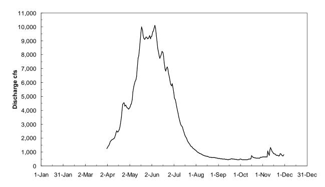
Figure 15. Average daily discharge from 1988 to 2013 for the South Fork of the Flathead River at the Twin Creek USGS gaging site.
