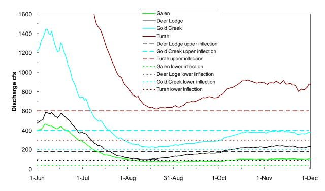
Figure 12. Average daily discharge from 1988 to 2013 at four USGS gaging sites on the UCFR with upper and lower inflection points associated with each gaging station.
