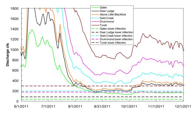
Figure 16. Daily discharge from 2011 (high flow year) at six USGS gaging sites on the UCFR with lower inflection points associated with each gaging station.
