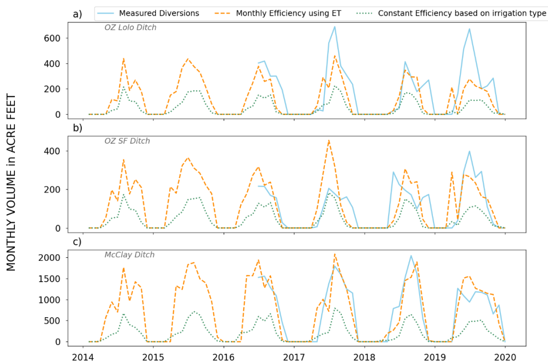
Figure A19. Graphs of diversion estimation results (orange dashed and green dotted lines) compared with measured diversions (blue solid line) for a) OZ Lolo Ditch, b) OZ South Fork Ditch, and c) McClay Ditch.
