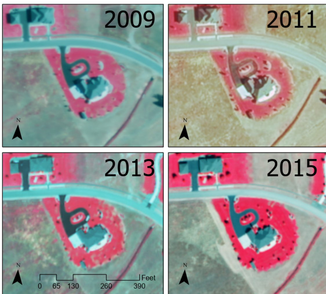
Figure A13. Example images showing multiple years of National Agricultural Imagery Program (NAIP) Color Infrared (CIR) aerial images at a scale of 1:2000. CIR displays green, growing vegetation as red pixels making it easy to identify watered areas. The extent of the red pixels within land parcels was used to estimate the area, in acres, of irrigated lawns in the Lolo Watershed. Notice the reoccurrence of red pixels over time from 2009 to 2015 suggesting that this area is indeed irrigated and has been in the past.
