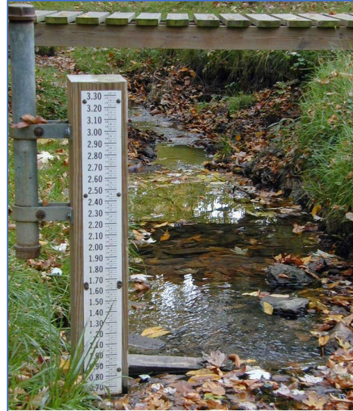
Figure 16: Staff gage coupled with a crest-stage gage (left side of photo).
