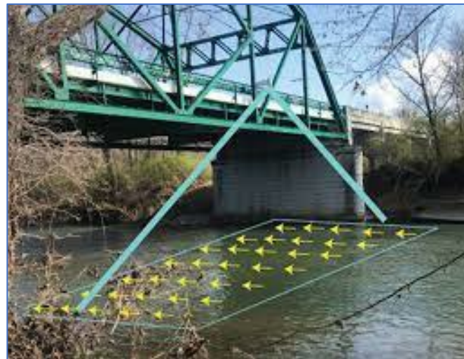
Figure 17: Large -Scale Particle-Image Velocimetry (LSPIV) uses video to capture particles on the surface of the water passing beneath the instrument.
