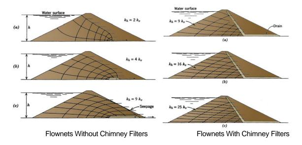
Figure 2 - Chimney Filters Provides Positive Phreatic Surface Control for Anisotropic Permeabilities
