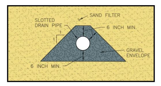
Figure 12 - Recommended Drain Pipe and Filter/Drain Configuration
