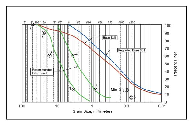
Figure 4 - Example of NRCS Filter Design Application
