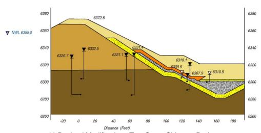
b) Revised Modification: Two Stage Chimney Drain
