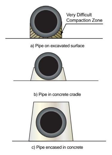
Figure 15 - Compaction Issues for Round Conduits
