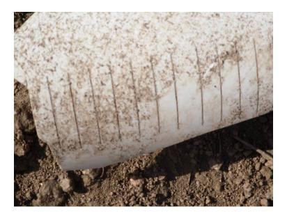
Figure 11 - Plugged Drain Pipe Slots
