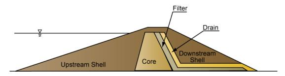
Figure 7 - Two-Stage Chimney Filter and Drain
