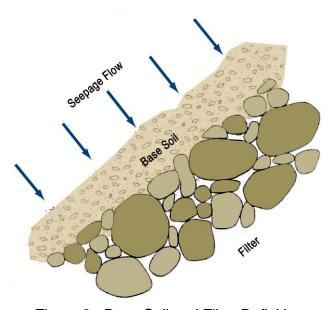
Figure 3 - Base Soil and Filter Definitions
