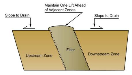
Figure 18 - Recommended Procedure to Prevent Contamination of Filter and Drain Materials
