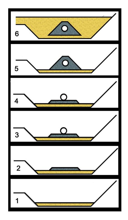
Figure 13 - Possible Sequence of Drain Pipe and Filter/Drain Construction
