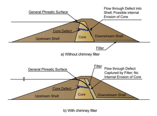
Figure 1 - Chimney Filters Provide Protection Against Core Defects
