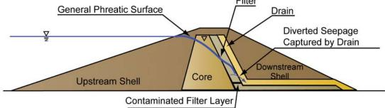
b) Two-stage chimney filter and drain
