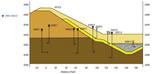
a) Original Modification - Single Stage Chimney Drain
