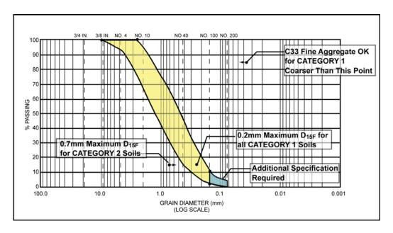
Figure 6 - ASTM C33 Fine Aggregate as a Filter
