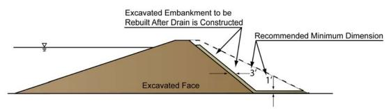
c) Inclined chimney placed against an excavated surface
