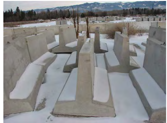
Concrete diversion blocks have a lifting ring and when placed in the streambed, the broad base keeps the block from tipping. Some site preparation may be necessary.
