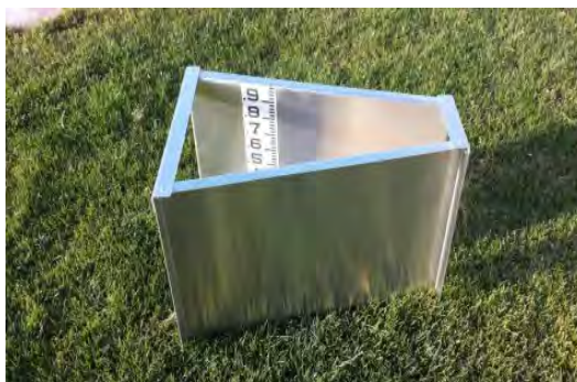
The Montana flume is a shortened version of the Parshall and must be free flowing (not backwatered).
