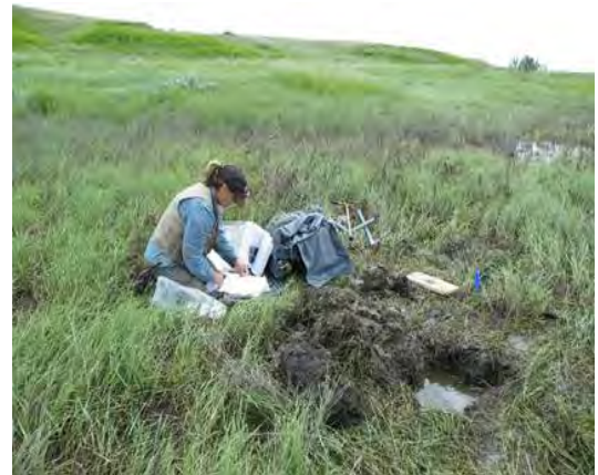
Soil pits are used to evaluate hydrology and hydric soil conditions.
