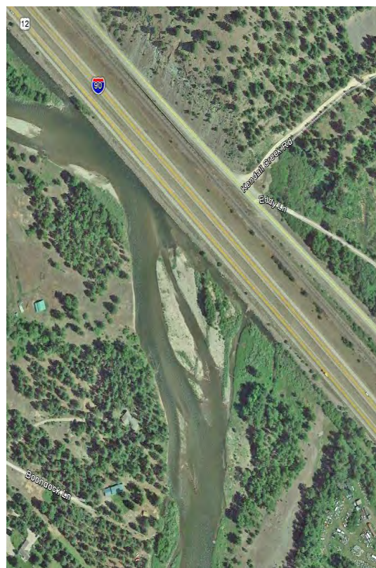
The river meander is moving downstream and recreating a floodplain. (Clark Fork 2015)
