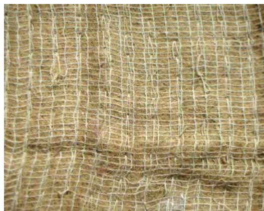
Finer coconut fabrics are frequently layered beneath the coarse coir fabric to prevent loss of fine soils.
