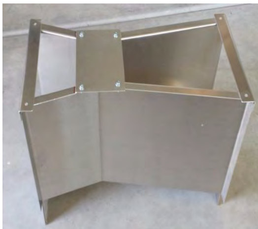
The cutthroat flume has similar characteristics to the Montana flume but can be corrected for submergence.
