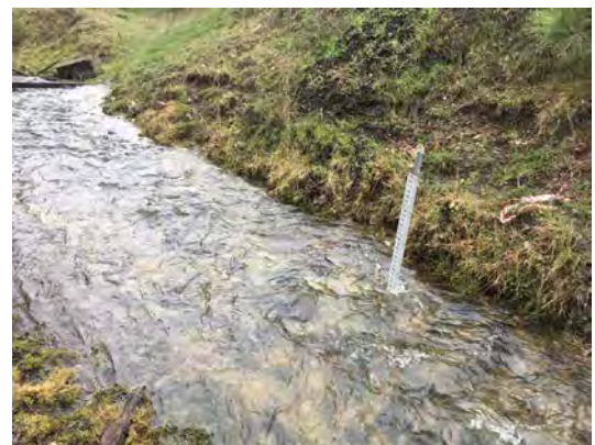
Stage-discharge relationships can be developed for open channels (or culverts) to monitor flow in ditches.
