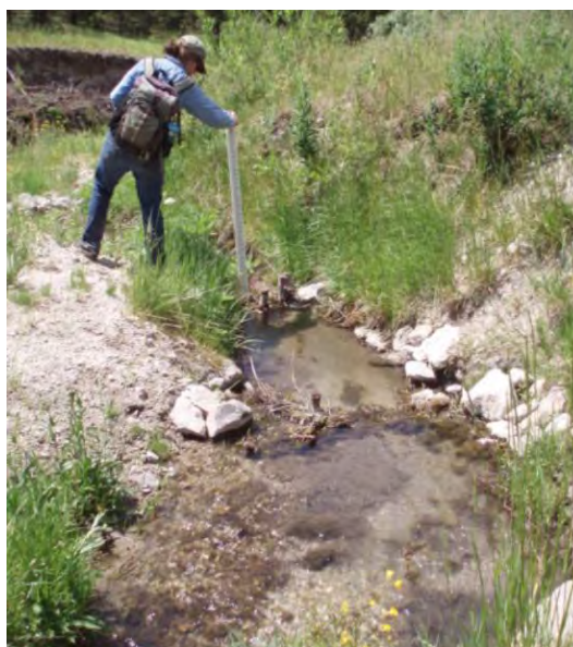
Incised channels may have stable stream bed elevations (Rosgen F type), or may be adjusting vertically (Rosgen G type).
