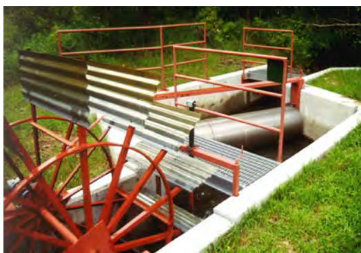
Large drum screens can accommodate a wide range of flows (from 5 to 50 cfs or more).
