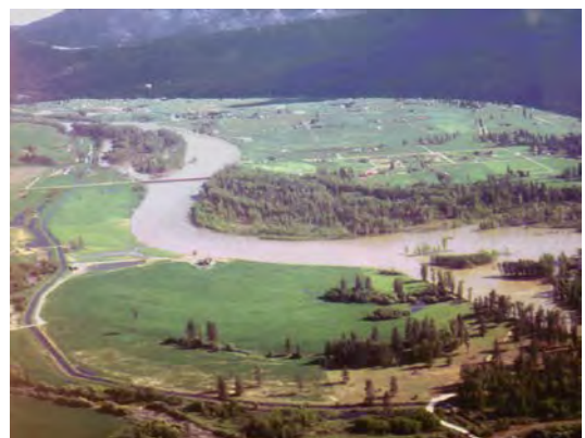
Replacement trees are colonizing the expanding point bar floodplain. The channel is moving several feet per year (20+ feet in 1997, alone), much to the dismay of the landowner.
