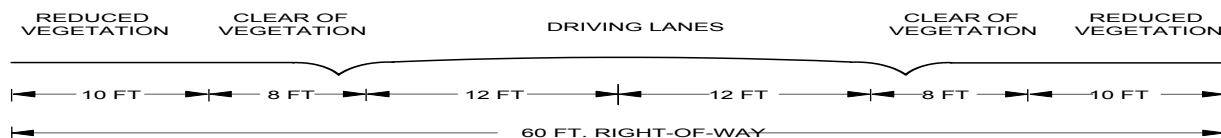
Figure 2 - Primary road right-of-way.
